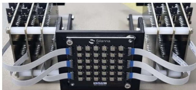
Figure 4: Emitter board with 6x driver boards.
