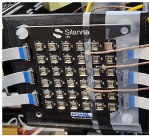
Figure 6: Emitter board with thermocouples .
